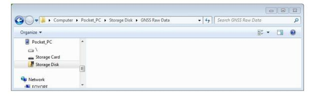
If raw data files are recorded to the SD card they will be found in the GNSS Raw Data folder on the SD card as shown in the following screen shot.
